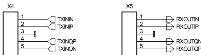
Pin header type connectors on the Myriad-RF board, provide analog IQ signals I/O.
